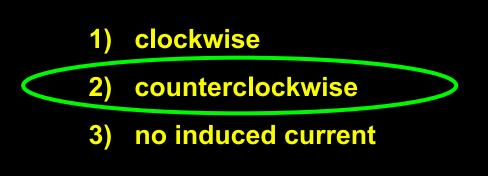
The *B* field points *into the page*. The flux is *increasing* since the area is increasing. The induced *B* field opposes this change and therefore points *out of the page*. Thus, the induced current runs *counterclockwise* according to the right-hand rule.
