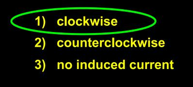
The **B** field into the page is disappearing in the loop, so it must be compensated by an induced flux also into the page. This can be accomplished by an induced current in the clockwise direction in the wire loop.
