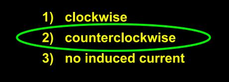
As the coil is rotated into the *B* field, the magnetic flux through it *increases*. According to Lenz' s Law, the induced B field has to oppose this increase, thus the new *B* field points to the right. An induced counterclockwise current produces just such a *B* field.
