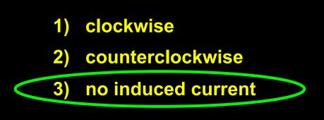
Since the magnetic field is uniform, the magnetic flux through the loop is not changing. Thus no current is induced.
